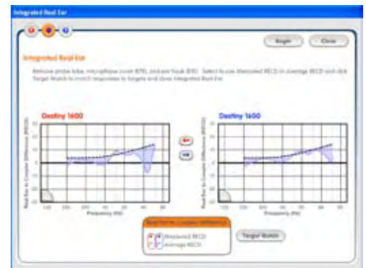
Figure 7. Integrated Real Ear window in Inspire OS, showing average RECD (black dashed line) and individual RECDs for right and left ears (blue line).
