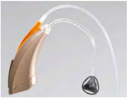
Figure 5. Probe tube attached to the Integrated Real Ear Measurement adaptor on a Zōn hearing instrument.
