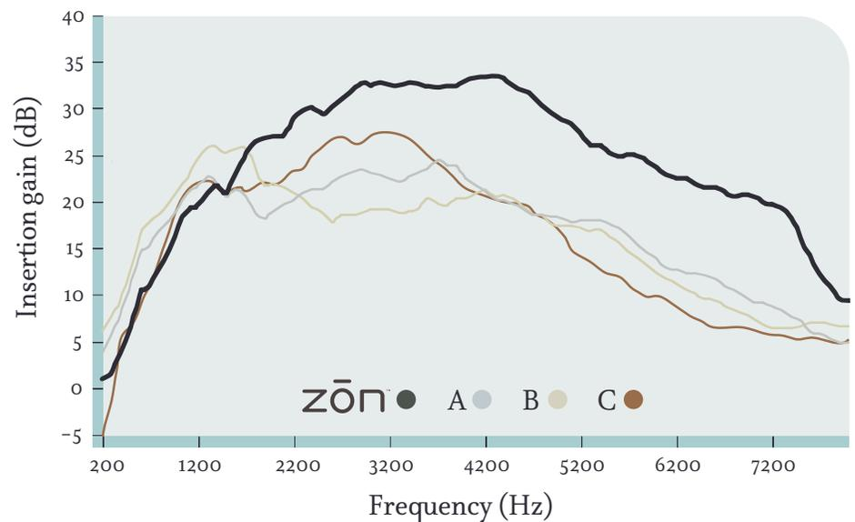
Figure 3. Mean insertion gain as a function of frequency for the Starkey Zōn and the three closest competitors.
