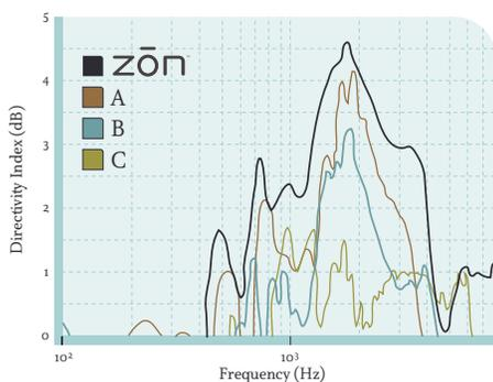
Figure 4. Directivity Index as a function of frequency for the Starkey Zōn and three competing RIC products.
