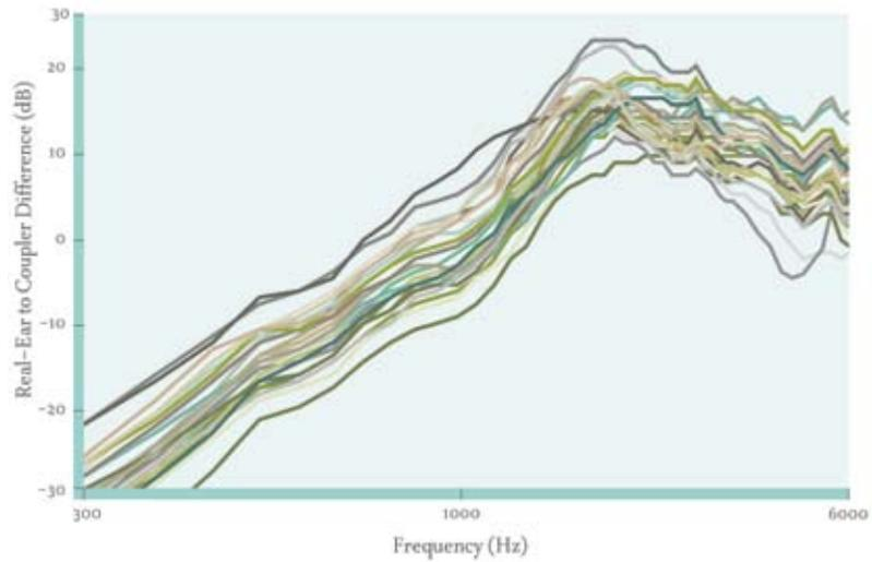
Figure 8. Thirty RECDs as a function of frequency, as measured using Integrated Real Ear Measurement in Zōn .7.
