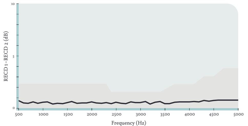
Figure 9. Mean difference between two RECDs as recorded using Integrated Real Ear Measurement in Starkey Zōn .7 as a function of frequency for 29 ears. The shaded area represents the range of variability in this measurement.
