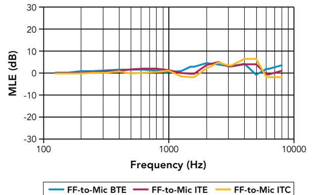
Figure 8. Microphone location effects for three hearing instrument styles.
