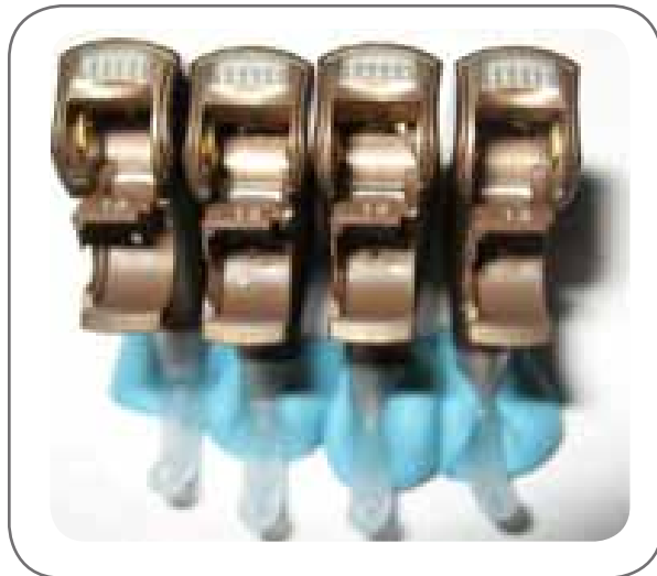
Figure 7: No corrosion was observed in the battery compartment or DAI contact area after two salt fog cycles.
