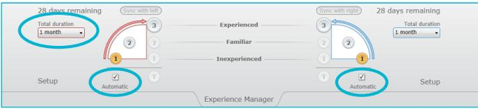
**Figure 1:** Inspire screen capture showing the Automatic Experience Manager feature enabled, as indicated by the checkmark on the screen, as well as six total duration options over which the automatic acclimatization process can occur.
