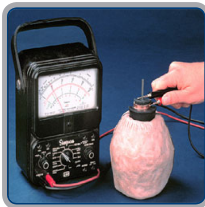
Figure 1: Estimated to be about 2,000 years old, the Parthian batteries produce an electrical current when filled with an electrolyte solution. As no written records exist, their use in ancient times can only be speculated on.
