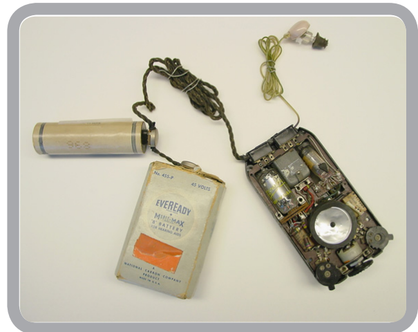
Figure 2: A typical body-worn vacuum tube hearing aid of the 1940s. The two batteries together are larger than the hearing aid itself.
