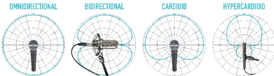
Figure 2. Various microphone sensitivity patterns.
