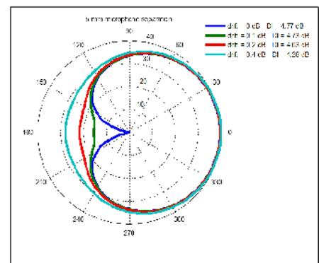
Figure 1. Impact of microphone drift on cardioid pattern directionality.
