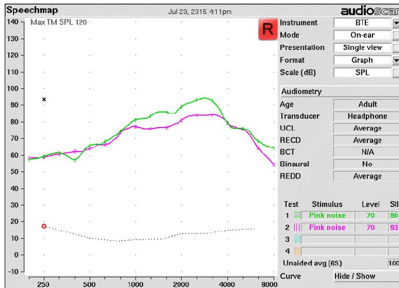
Figure 4. Speechmap using pink noise to show directional microphone benefit using a Z Series RIC in Fixed Directional mode.
