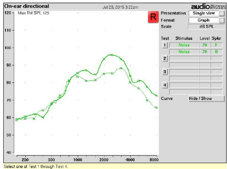
Figure 3. On-Ear directional microphone test results using a Z Series RIC in Fixed Directional mode.
